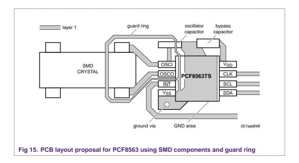
**Remark**: Take precautions when cleaning PCBs containing tuning fork crystals using ultrasound. The resonance vibration may damage the crystal. Consult the supplier of the crystal in case of doubt.
