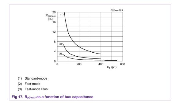
Below  $R_{p(max)}$  is calculated for both Standard-mode and Fast-mode  $I^2C$  bus. The result has been rounded down to E6 standard values.
