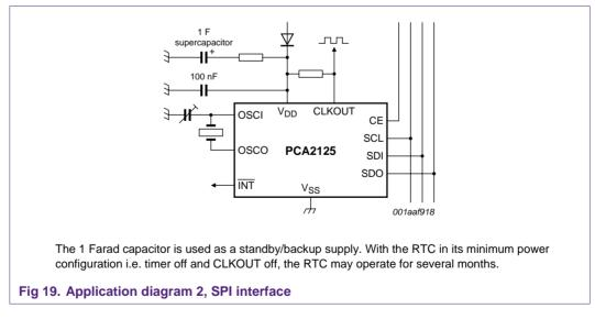
**Remark**: CLKOUT and INT are open drain outputs. If a pull-up resistor is used, it should not be connected to voltages higher than the maximum operating voltage as specified for the RTC. If the outputs need to be used to switch signals connected to a higher potential, it is necessary to use an external transistor.
