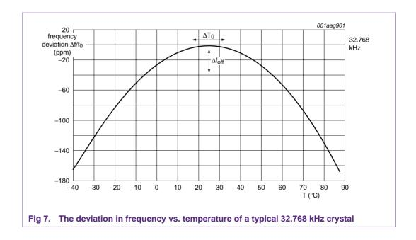
The frequency of a typical crystal at a specific temperature T is given by:
