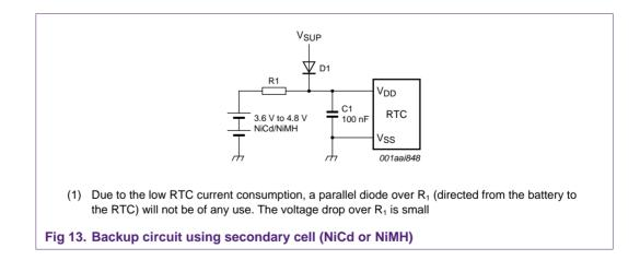
The capacity of a battery is expressed as C. The charge or discharge current can now also be expressed in relation to the capacity of the battery. Assume a battery with a capacity of one ampere-hour (1 Ah). A discharge current of C/10 now equals 1 Ah / 10 h = 100 mA. The recommended charge current is also specified as a fraction of C.
