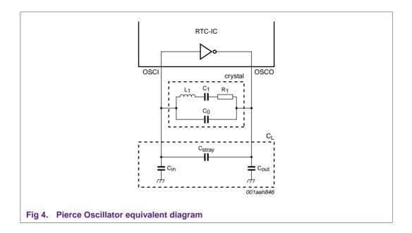
The inverting amplifier (with feedback resistor, and drive resistor which are not included in Fig 4) is incorporated within the integrated circuit device. On the other hand, the quartz crystal is a discrete device external to the integrated circuit. In the PCF85x3, PCA8565 and PCF2123, PCA2125 the output capacitor  $C_{OUT}$  is integrated on the integrated circuit. PCF8563A, PCA8565A and PCF2123 also include  $C_{IN}$ , see Table 3 for overview.
